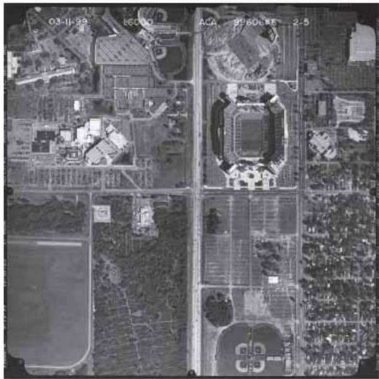
Aerial photograph taken at 910 m above ground, scale 1: 6,000
