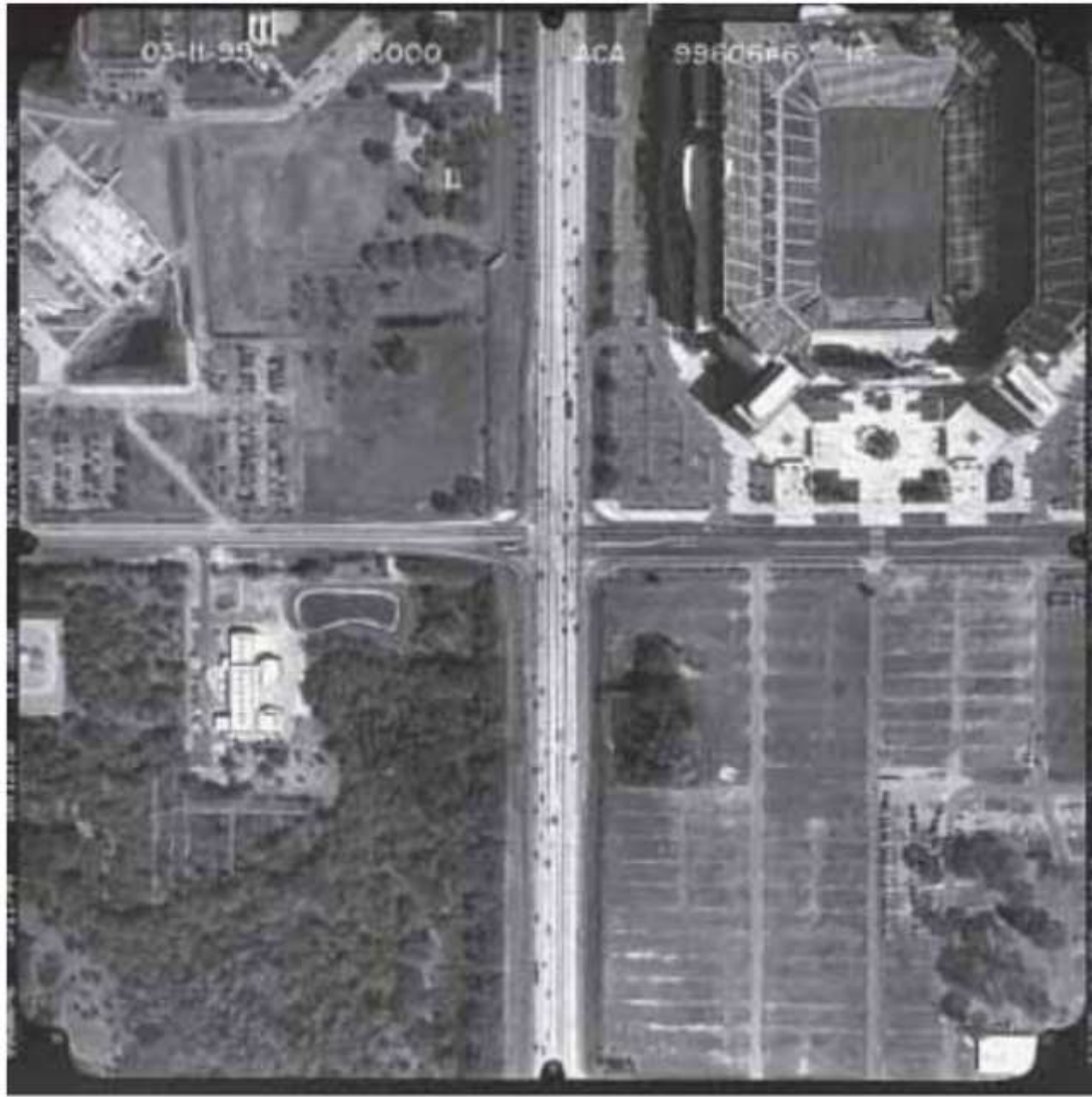
Aerial photograph taken at 460 m above ground, scale 1: 3,000
