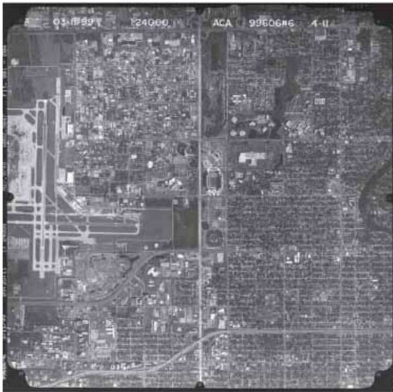
Aerial photograph taken at 3660 m above ground, scale 1: 24,000
