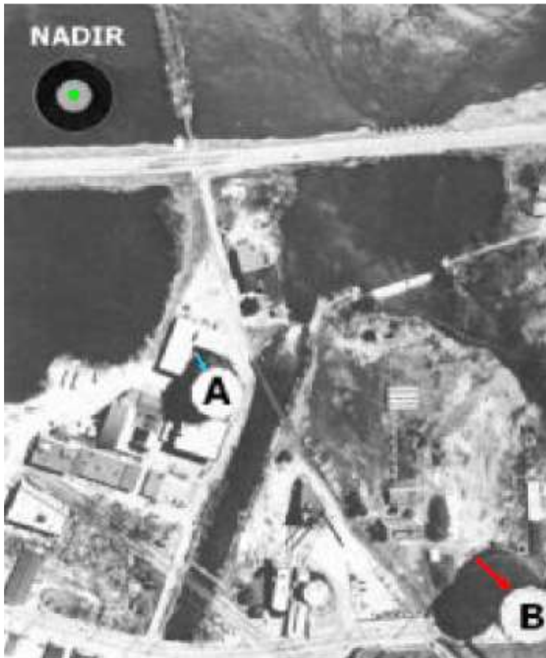
Relief displacement from Nadir (enlarged)
