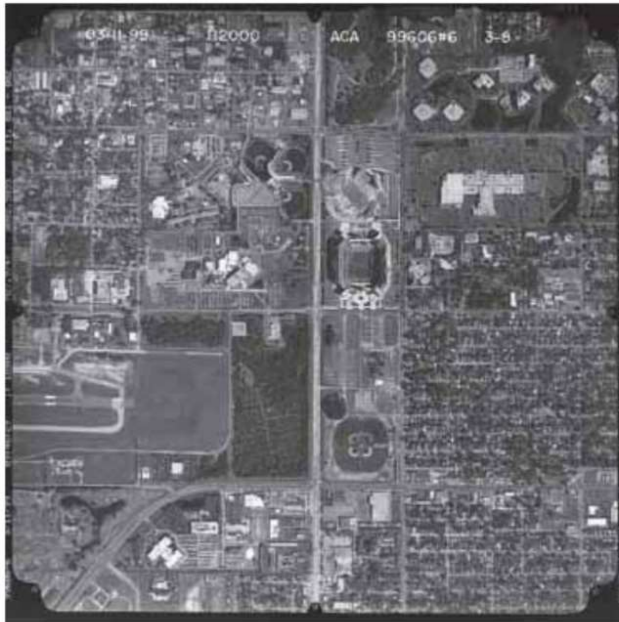
Aerial photograph taken at 1830 m above ground, scale 1: 12,000
